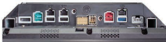
Selectable and upgradeable SurePorts enable retailers to use existing devices and connect customer or employee devices
